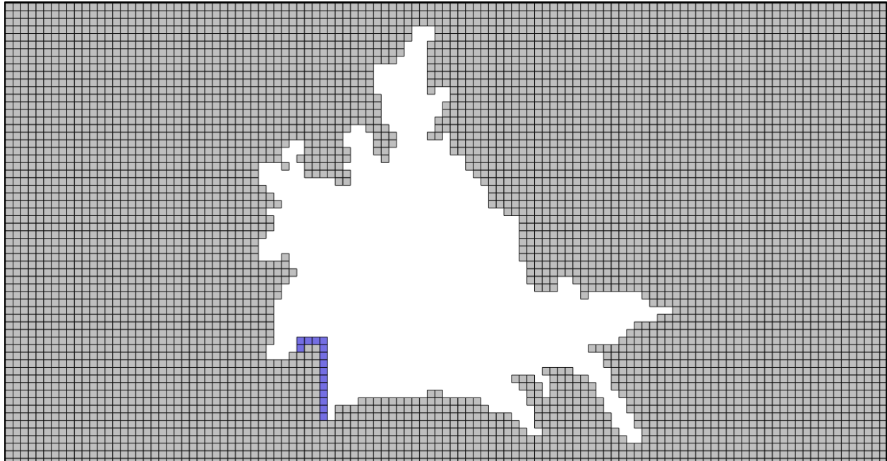
Figure B-5. Constant-head boundary cells used to simulate Deer Creek Reservoir groundwater level control.
